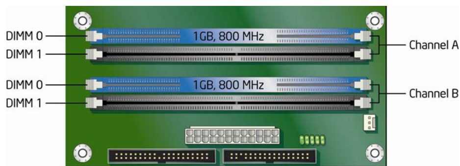
Figure 13. Dual Channel Memory Configuration with Two DIMMs
